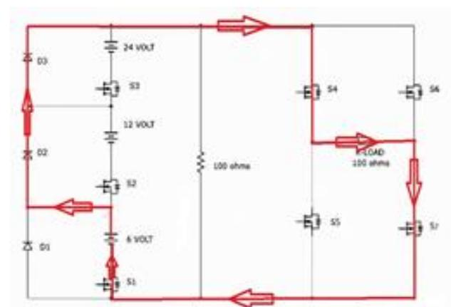
Fig. 4. Modes of operation for 6V for positive half cycle
