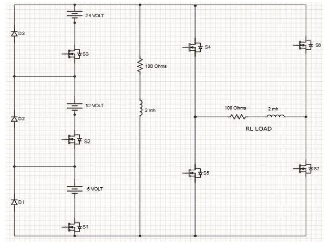
Fig. 7. Circuit diagram of 15 level with R-load
