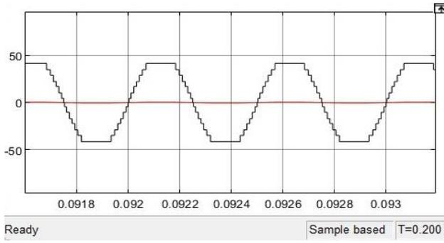
Fig. 10. Simulation output of R load at 2000Hz(42V)
