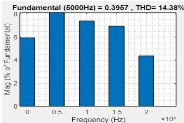
Fig. 27. FFT analysis of RL load at 5000Hz (42V)
