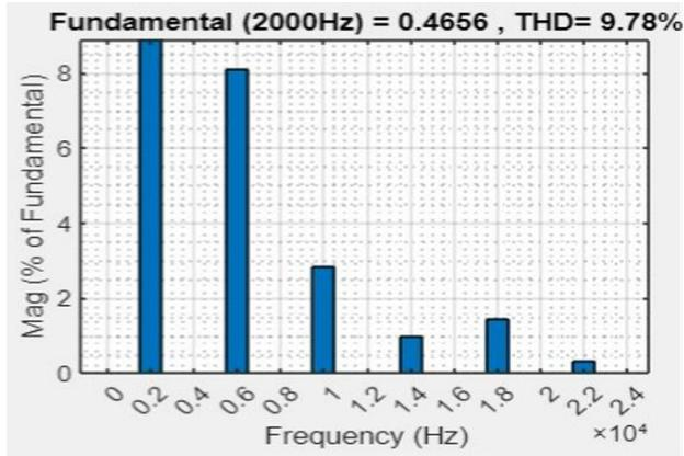
Fig. 11. FFT analysis of R-load with 2000 Hz(42V)
