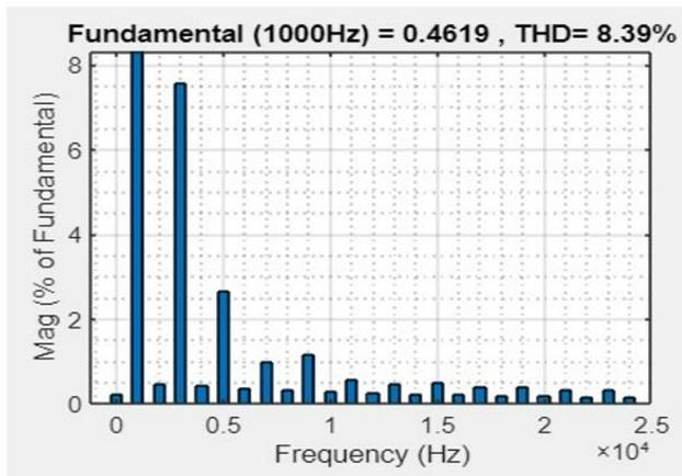
Fig. 19. FFT analysis of RL-load with 1000 Hz (42V)
