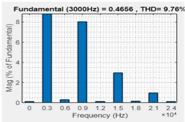
Fig. 13. FFT analysis of R-load with 3000 Hz (42V)
