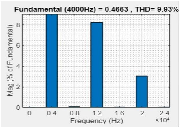
Fig. 15. FFT analysis of R load at 4000Hz (42V)
