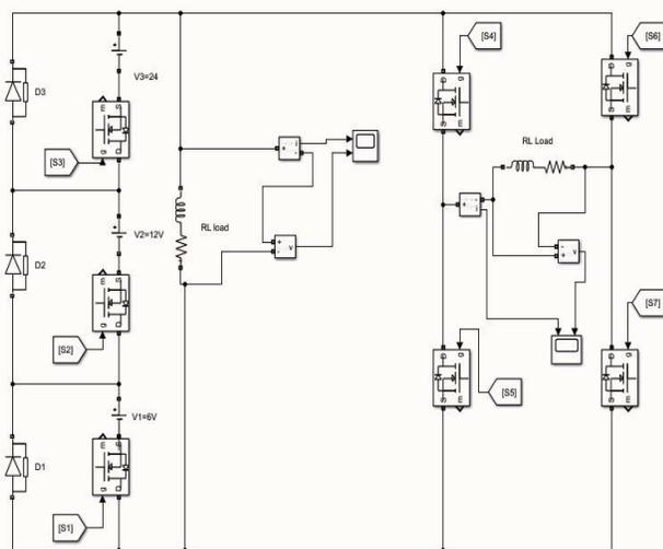
Fig. 6. 15-level inverter circuit with RL load
