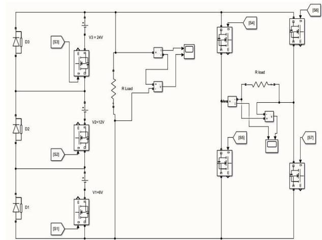
Fig. 2. 15-level MLI with R-load
