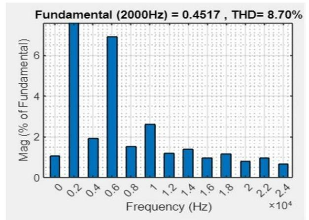
Fig. 21. FFT analysis of RL load at 2000Hz (42V)
