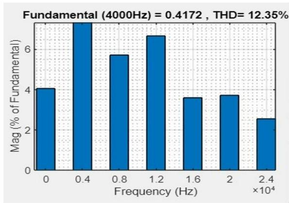
Fig. 25. FFT analysis of RL load at 4000Hz (42V)
