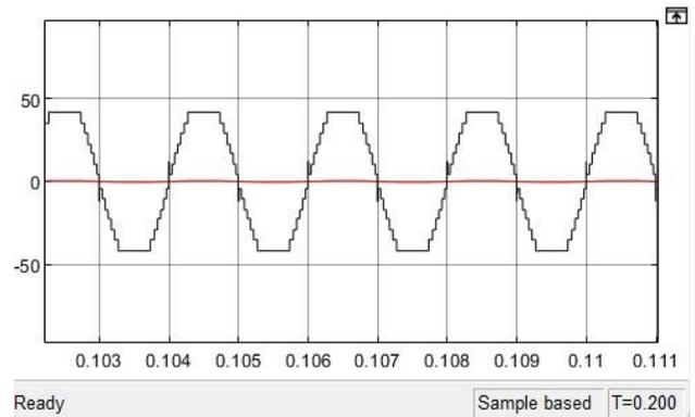
Fig. 22. Simulation output of RL load at 3000Hz (42V)
