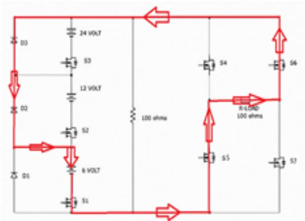
Fig. 5. Modes of operation for 6V for negative half cycle
