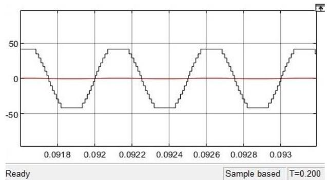
Fig. 8. Simulation output of R load at 1000Hz (42V)
