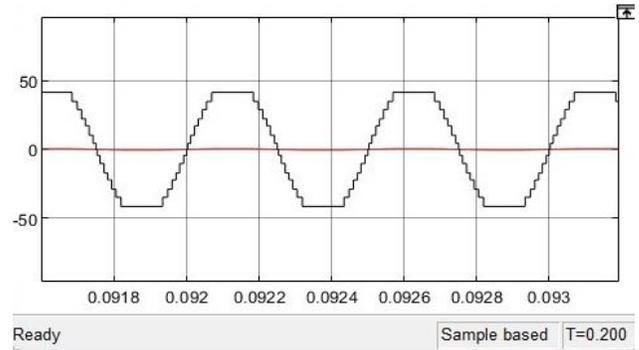
Fig. 14. Simulation output of R load at 4000Hz (42V)
