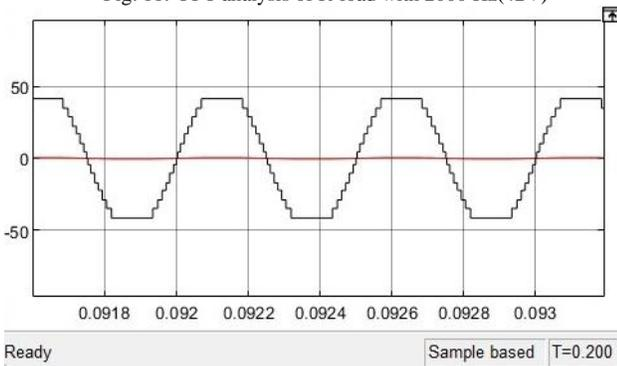
Fig. 12. Simulation output of R load at 3000Hz(42V)
