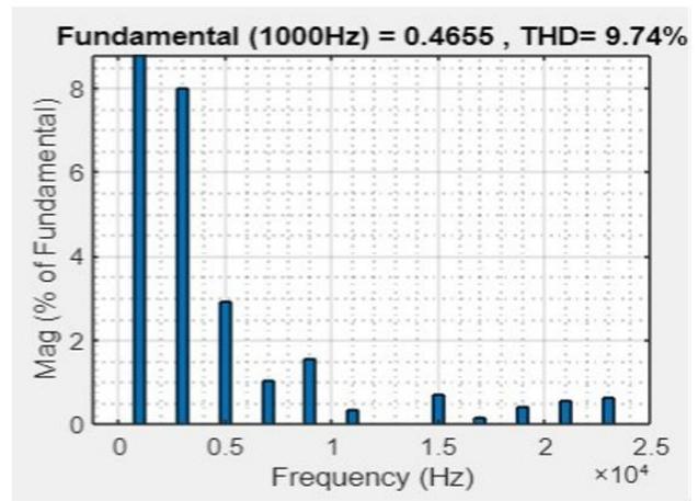
Fig. 9. FFT analysis of R load at 1000Hz(42V)
