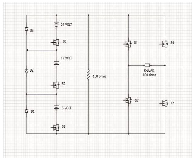
Fig. 3. Circuit diagram of 15 level with R-load
