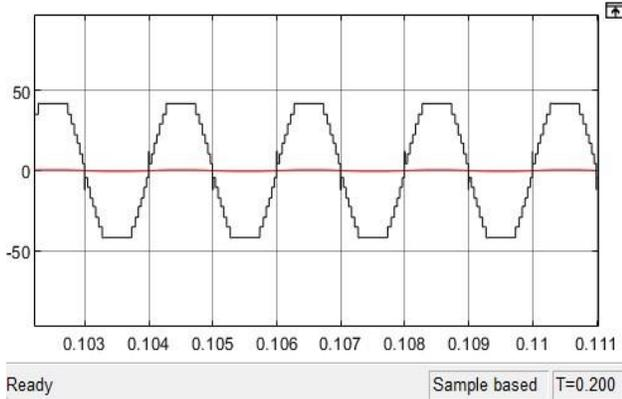
Fig. 18. Simulation output of RL load at 1000Hz (42V)
