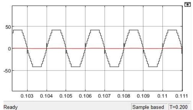
Fig. 24. Simulation output of RL load at 4000Hz (42V)
