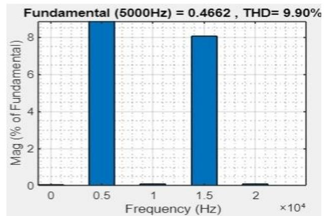
Fig. 17. FFT Analysis of R load at 5000Hz (42V)
