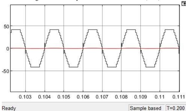
Fig. 26. Simulation output of RL load at 5000Hz (42V)
