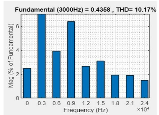
Fig. 23. FFT analysis of RL load at 3000Hz (42V)
