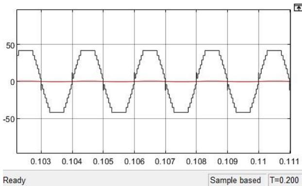
Fig. 20. Simulation output of RL load at 2000Hz (42V)
