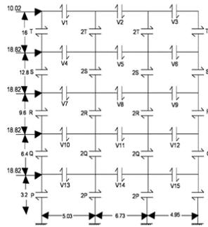
Fig. 3. Wind forces acting on a frame
