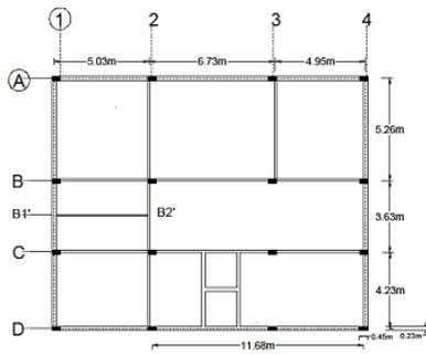
Fig. 2. Beam column lay out of one flat of the building
