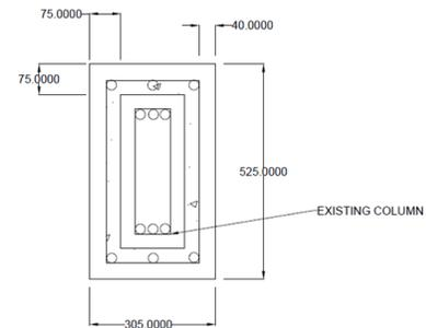
Fig. 4. Layout of Retrofitted Column
