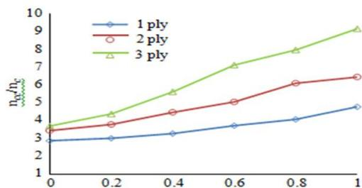
Fig. 5. Corner radius effect on strain improvement ratio
