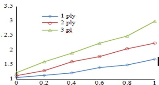
Fig. 4. Effect of corner radius on strength enhancement ratio
