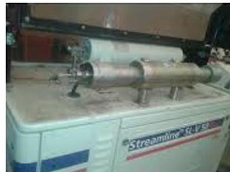
Fig. 4. KMT Streamline SL-V 50- high pressure pump
