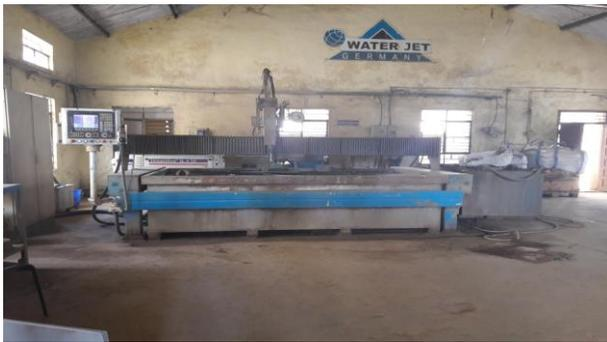
Fig. 1. CNC controlled abrasive water jet machine
