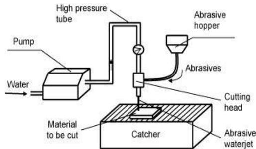
Fig. 5. Schematic diagram of basic principle of AWJM
