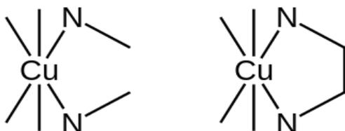
Fig. 2. Cu<sup>2+</sup> complexes with non-chelating Methylamine on the left and chelating Ethylenediamine on the right
