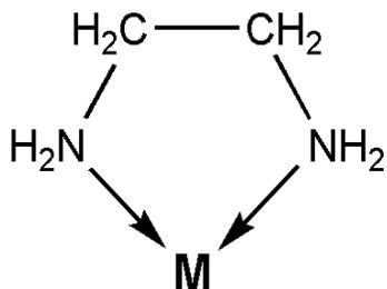
Fig. 1. Chelating structure, where M is the metal; M can be substituted for Lead, Arsenic and other metals
