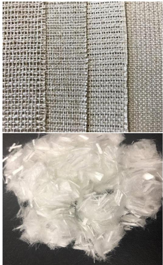
Fig. 2. Textile reinforcement
