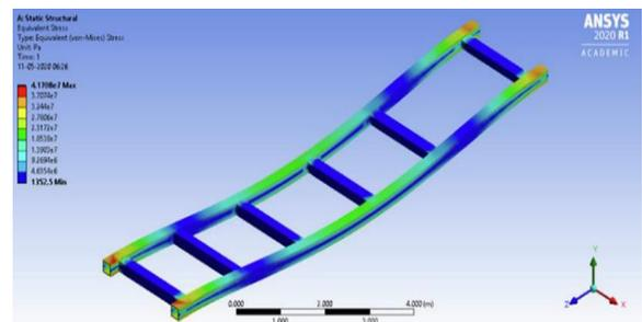
Fig. 5. Equivalent Stress of Aluminium 6061-T6 frame
