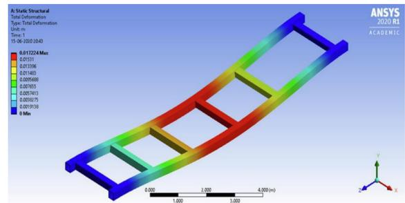
Fig. 6. Total deformation of Aluminium 6061-T6 frame
