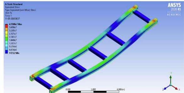
Fig. 7. Equivalent stress of Aluminium 7075-T6 frame
