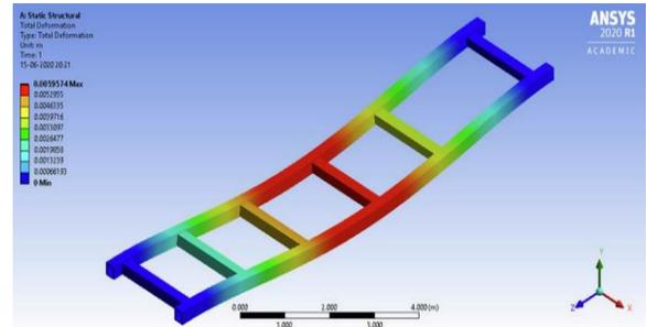
Fig. 4. Total deformation of steel frame
