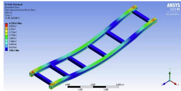
Fig. 3. Equivalent stress of steel frame
