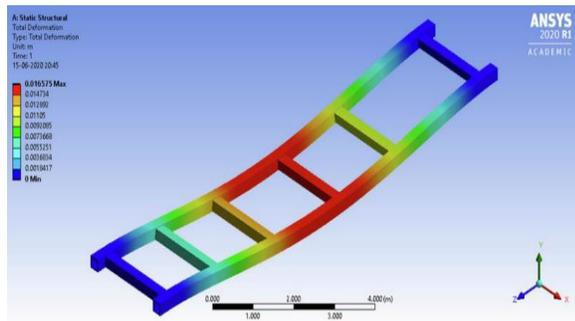
Fig. 8. Total deformation of Aluminium 7075-T6
