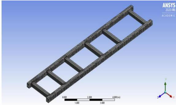
Fig. 2. Meshed model of the chassis frame
