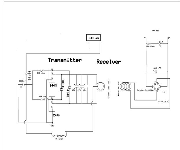
Fig. 2. Circuit diagram of the project
