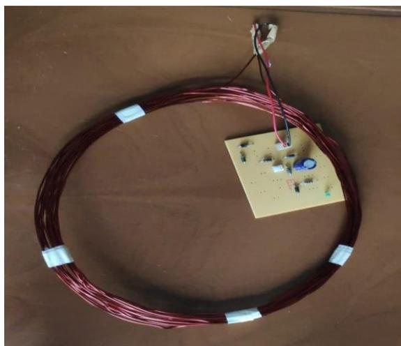
Fig. 4. Receiver coil of WPT
