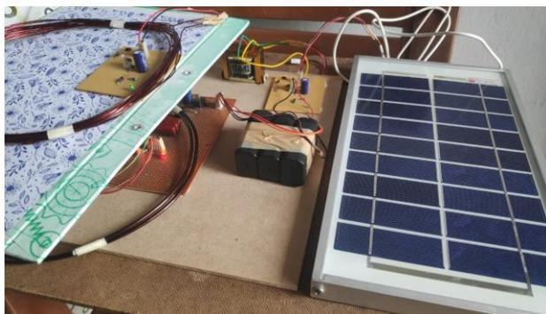
Fig. 5. LED glows in the receiver coil
