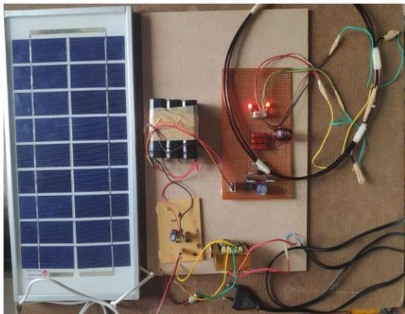
Fig. 3. Transmitter coil of WPT
