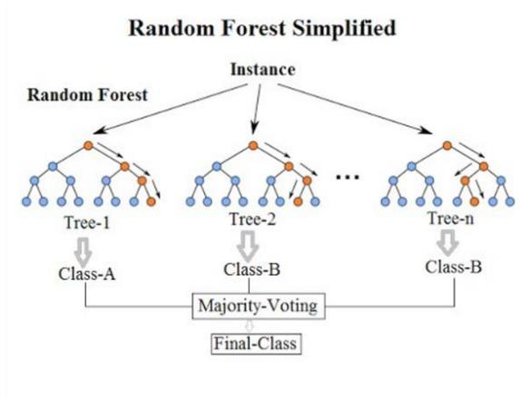
Fig. 5. RFC algorithm
