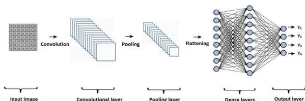
Fig. 3. CNN architecture
