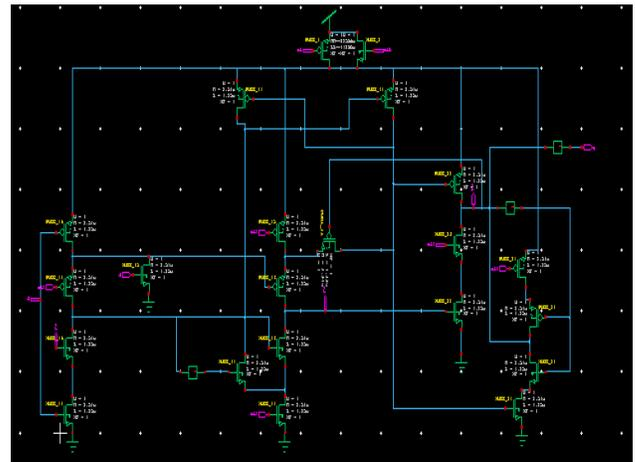
Fig. 3. Schematic of Proposed Flip Flop in S-Edit
