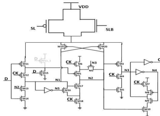
Fig. 1. Schematic of Power Gated Flip Flop
