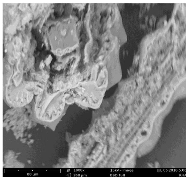
Fig. 2. SE image of the thermally treated rice husk ash (RHA)
