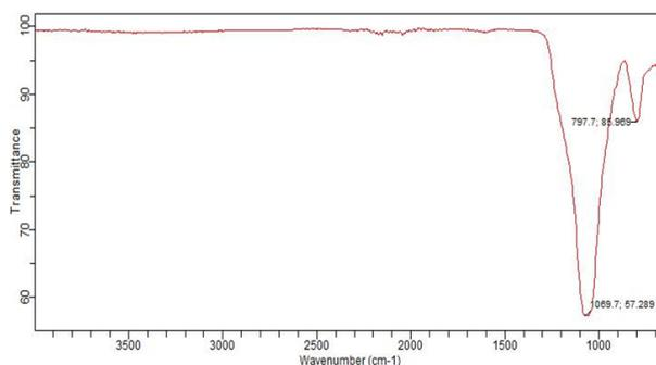
Fig. 3. FTIR spectrum of the thermally treated rice husk ash (RHA)
