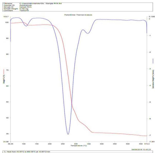
Fig. 4. Thermogravimetric curve of the thermally treated rice husk ash (RHA)
