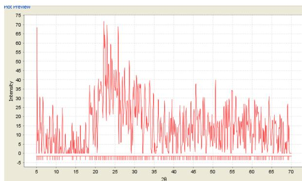
Fig. 1. X-ray diffraction pattern of the thermally treated rice husk ash (RHA)
