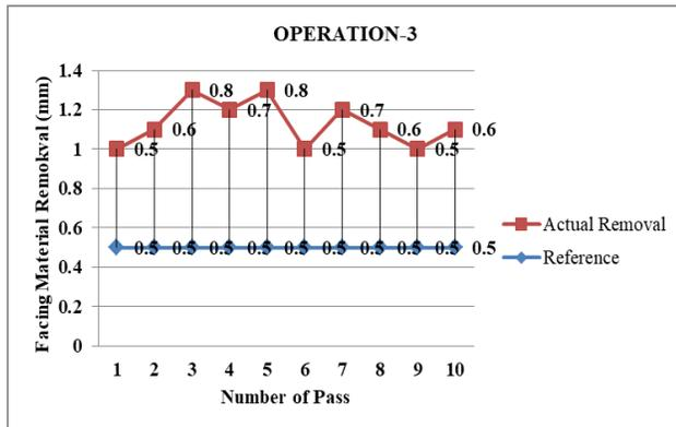
Fig. 6. Variation of material removal in Operation-3
