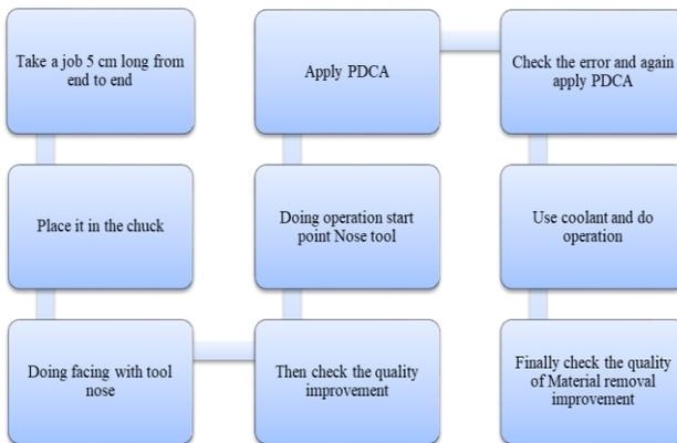
Fig. 3. Flow chart of operation
