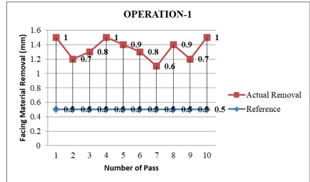
Fig. 4. Variation of material removal in Operation-1
