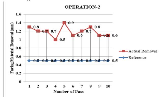
Fig. 5. Variation of material removal in Operation-2
