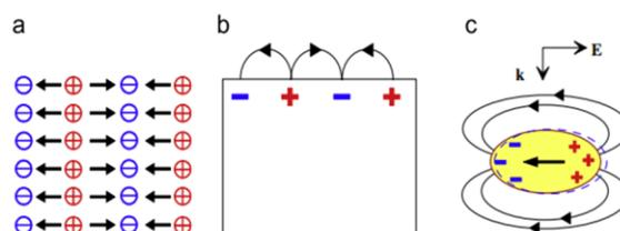
Fig. 1. Schematic of (a) surface propagating (b) and surface localized (c) plasmons. The dashed line shows the electron cloud displacement [21]
