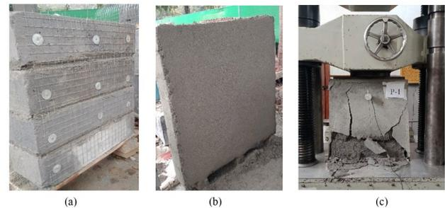
Fig. 4. Samples (a) Strengthened (b) Without strengthening (c) Testing
