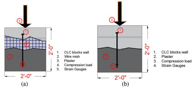
Fig. 3. Samples (a) Strengthened (b) Without strengthening
