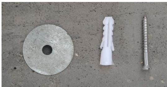
Fig. 2. Washer, Plug, Screw
